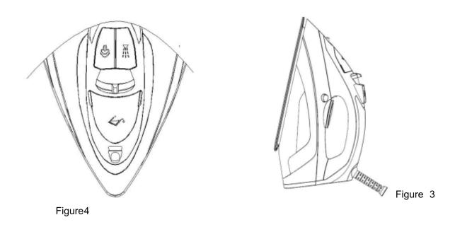
5. Once soleplate temperature has reached the preset temperature, indicator light will be off, then set steam button to your desired steam output or dry position and begin ironing.
